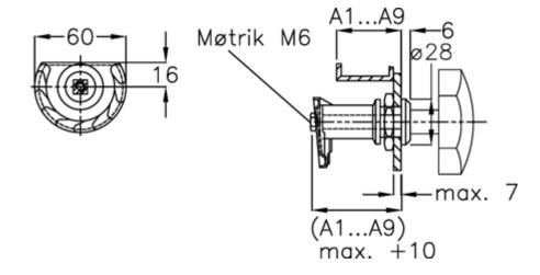
Door + frame thickness = 32-40 Measure type = A4
